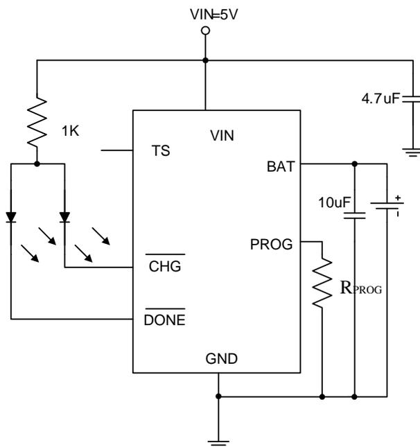
注：充电电流  $I_{BAT} = (1.2/R_{PROG}) * 1000$ ;
