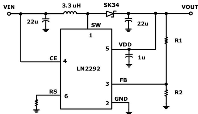
$$V_{OUT} = V_{FB} \times \left(1 + \frac{R1}{R2}\right)$$
